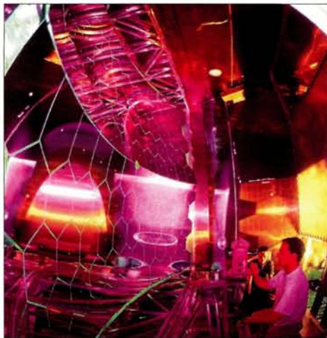
Mirrors for the Ring Imaging Cherenkov detectors of the COMPASS experiment at CERN. COMPASS is the latest in a long line of spin-sensitive experiments using CERN high-energy muon beams.
