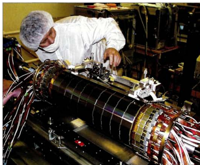
The CLEO silicon strip vertex detector during construction. The double-sided silicon wafers are clearly visible. These will surround the beam pipe.
