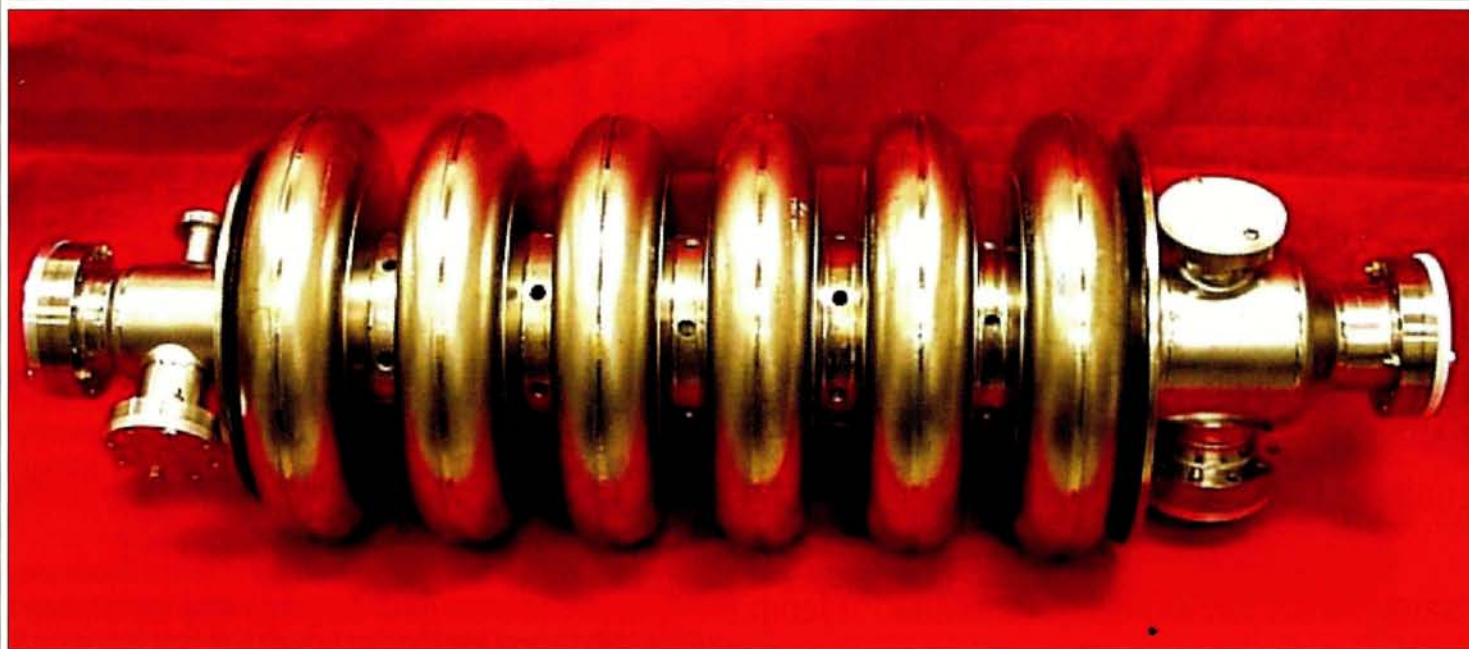
State of the art – an 805 MHz prototype six-cell solid niobium cavity ( \beta = 0.61 ) built at the US Jefferson Laboratory for the Spallation Neutron Source that is under construction at Oak Ridge and for which the Jefferson Laboratory is responsible for cavity production in close collaboration with Los Alamos. The total length of the device is 107 cm and the active length (cells only) is 67.5 cm. The stiffener rings with holes for helium passage can be seen between the cells.
